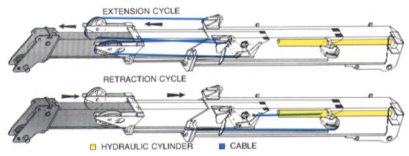
EXTENSION CYCLE - As the mid-section is extended by the telescope cylinder, the fly section is pulled out of the mid-section in direct proportion by a % in. (22mm) cable. The extension cable has a safety factor of 3.5 to 1 (6 to 1 with international version and 11/a in. (29mm) dia. cable) and is attached with threaded connections at base section and retained on either side of the sheave segment by swaged collars. This prevents the boom from retracting should the cable break.
